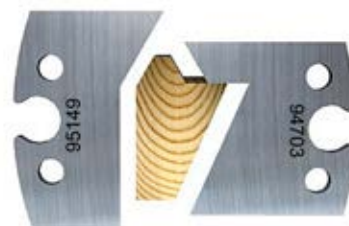
Shadow moulding, 21x33 mm
