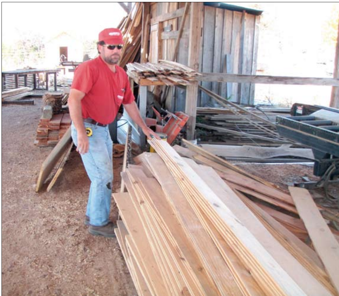
The Arkansawyer sorts through some oak tongue and groove flooring that he processed on the PH260 planer/moulder. He says that many customers are willing to pay more for "character" lumber that would be downgraded or rejected by commercial lumber buyers.
