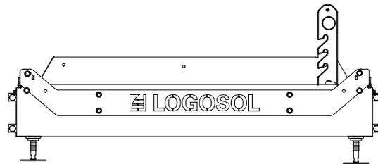
**3.** Use the accessory SMART Turner when rolling a log on the log bed. Centre the log on the log bed and roll it up against the log supports. Check the position of the log on the log bed. To be able to cut through the whole length of the log, the log should not protrude past the last cross bunk.
