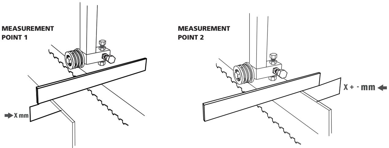
If the measurements differ, turn the adjusting bolts on the blade guide until the measurements are the same at both measurement points. One method to facilitate adjusting, is to use the value from measurement point 1, compare it with the value from measurement 2 and then, by raising or lowering the blade guide, adjust half the difference at measurement point 2. When the blade is parallel to the rails, repeat the adjustment steps on the other blade guide roller.
