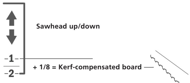
On the crank shaft, there is an opening where you can see numbers on a scale. This scale has eight steps, where each step is 1/8". **TIP:** When a board is cut above the blade, you have to compensate for the kerf, i.e. 1/8". The wood piece below the blade never needs to be kerf compensated. It has the same measurement that is shown on the absolute scale on the front leg of the carriage.
