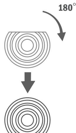
*Rotate the log 180° so that the freshly sawn surface rests on the log bed*
