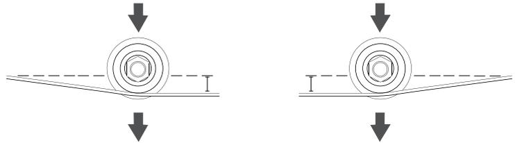
The blade guides can adjust the angle of the blade, measured in the direction of the cut, by adjusting the top and bottom adjusting bolts.
