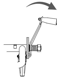
Once the handle is in good working order, you bend the lock washer to secure the lock nut in position.
