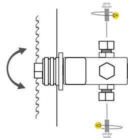
The blade guide can be adjusted inwards and outwards by pulling or pushing its shaft after the adjusting bolts have been loosened. The back of the blade should be approx. 3-5 mm from the rear edge of the blade guide roller.
