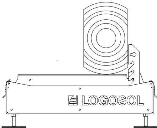
*Rotate the log 90° so that one of the freshly sawn sides rests flat against the log supports, and then clamp the log in position.*
