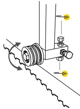
The blade guides must be adjusted so that they are parallel to the back of the blade. This is done by adjusting the outer and inner adjusting bolts. It is crucial that the blade guides run parallel to the blade. Be careful to adjust this correctly.
