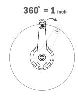
The locking mechanism of the crank is divided in eight steps per revolution. Each step moves the sawhead by 1/8", and one full revolution represents 1".
