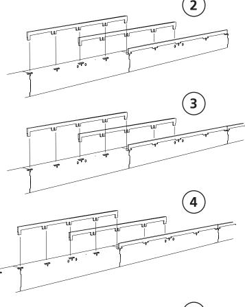
The last short rail section should be fitted the same way as the first one. See the first step of assembly on page 36.
