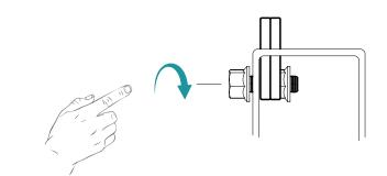
Tighten the bolt joints fingertight!
