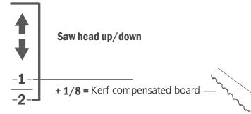
On the crank shaft, there is an opening where you can see numbers on a scale. This scale has eight steps, where each step is 1/8". **TIP:** When a board is cut above the blade, you have to compensate for the kerf, i.e. 1/8". The wood piece below the blade never needs to be kerf compensated. It has the same measurement that is shown on the absolute scale on the front leg of the carraige.
