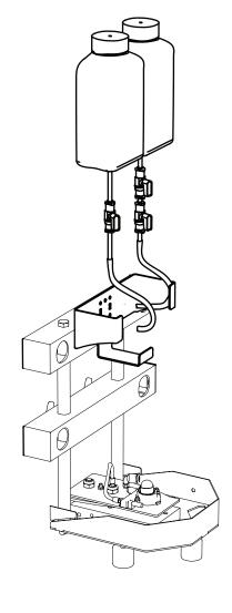
Connect the bottles to their respective valves. Note that the water bottle has two valves, one for adjusting the flow and one for turning the flow on or off. The oil bottle is to be connected to the oil pump.
