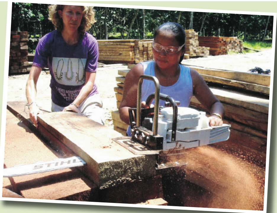
• Making planks from discarded cutoffs with the Timberjig in Ecuador.
