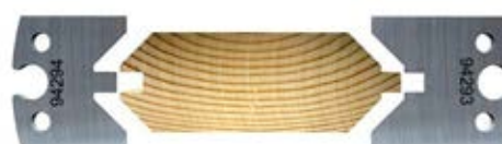
Double 45° Chamfered panel
