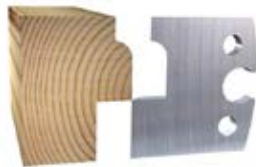
Moulding knife: 94364HSS Mating moulding knife: 94365HSS
