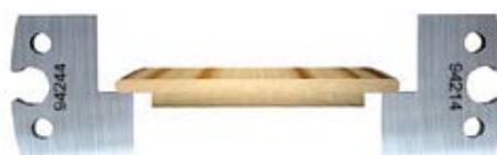
Double groove panel, joining piece
