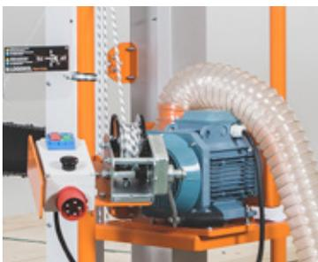
When you are cutting, the electric motor is protected by temperature sensors.
