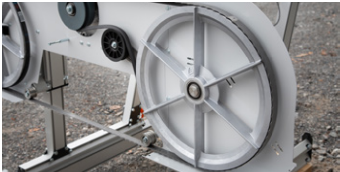
Band wheels with fan blades, cools the blade and keeps the cover clean.
