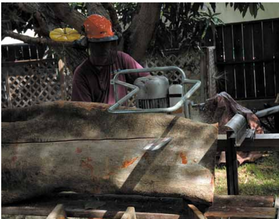
Darrell with M7 and electric powerhead cutting Koa log.
