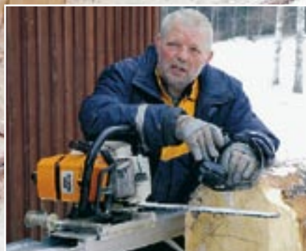
Poul Nielsen (inset) with an extraordinary sawmill! Three and a half M7s were the only way that the 17-metre long, ruler straight beams could be cut out for use in rebuilding the church tower.
