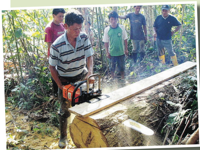
• Making planks from discarded cutoffs with the Timberjig in Ecuador.
