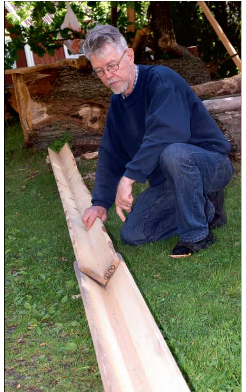
"The ridges and the rain gutters are made in sections," explains Carl Gustaf Olofsson and demonstrates that the lengths can be adjusted without using a saw.
