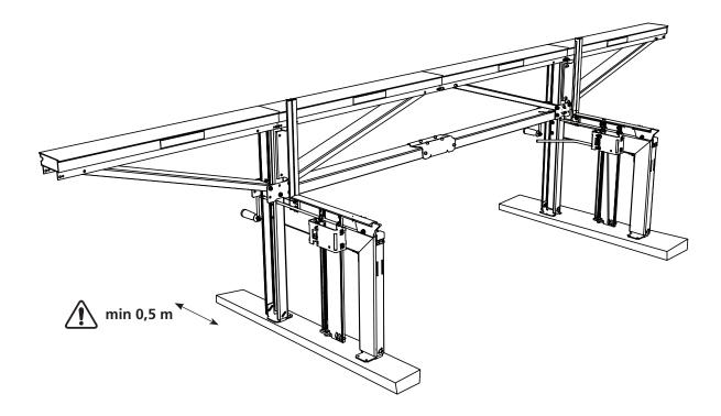
When the sawmill is placed directly on the ground, The surface must be firm and level enough to drive a car on.
