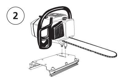
Fit the Logosol nuts through the track in the carriage. Tighten the chainsaw into place by using the chainsaw's guide bar nuts under the plate.
