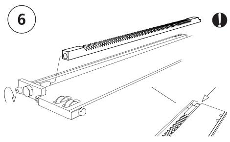
Make sure that the end of the ratchet bar does not extend over the end of the lifting beam, since this makes it impossible to assemble the log bed. The ratchet bar is normally slightly bent towards the toothed side. When screwing it into place, it will get a tight fit against the lifting beam by the tension created.
