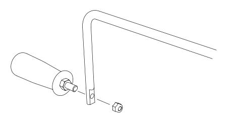
Note that the end of the line has to be fitted in the locking ring before assembly.
