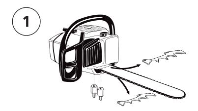
Unscrew the two guide bar nuts from the chainsaw and remove the guide bar cover.
