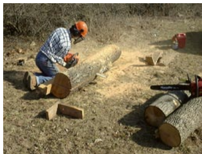
Ted Christiansen with his Logosol Timberjig. This guide rail is made from a 2"x6"x10' plank.
