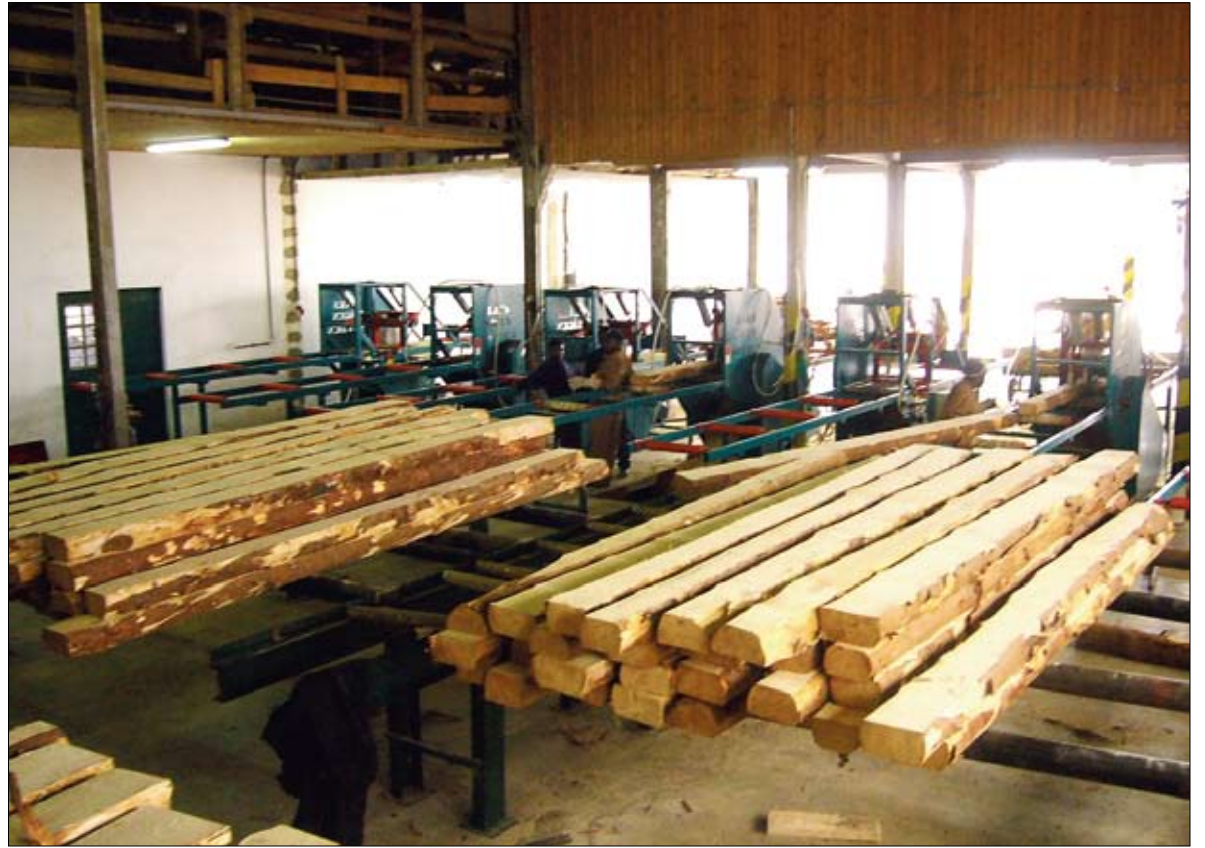
Eight Laks saws turned a wrecked pine plantation into profitable forestry with record-low investment costs. The sawmill was started up in 2005, and today it produces 1 060 000 cubic feet per year.
