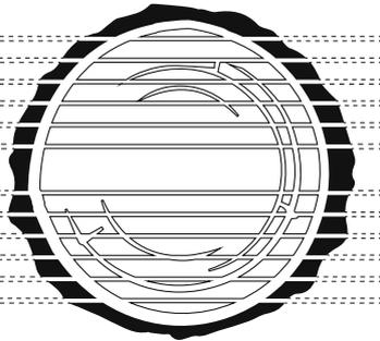
When you are going to slice a log, it is good if you first saw off a thin butt cut and then turn the log downwards so that the log rests on a flat surface. This ensures that the log does not move between the cuts and you will get nice, even, thick boards. Flip the log as you approach the center.
