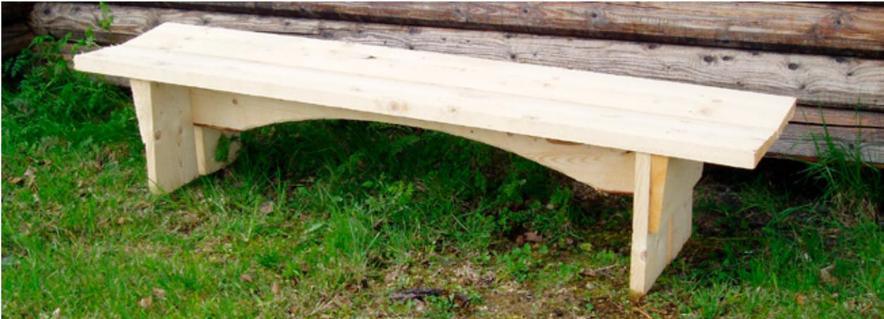
From log to finished bench takes about an hour. Use a chain sawmill, tape measure, carpenter square, hammer and nails - and don't be unnecessarily careful, it will turn out really great!
