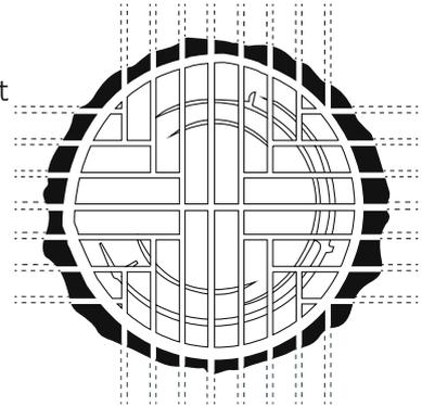
Start by sawing the log in the middle, but do not saw all the way through. Turn the log 90°. Now saw through the entire log. Then break the parts apart so that you get four quarters.
