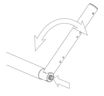
Loosen the upper tubular arm bolts. Adjust the arm to the desired height. Then tighten the bolts.
