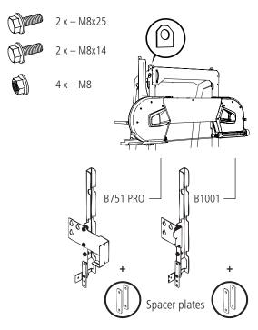
If you have this model, all parts should be pre-assembled and then hung up on the sawmill.
