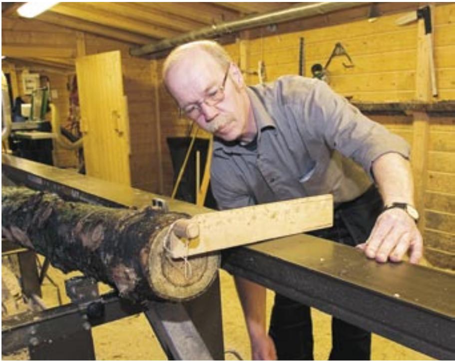
Pelle Boström, Sweden, demonstrates how the setting gauge works. When it lies like this on the guide rail, the sawn surface will be exactly where the nail is fastened.
