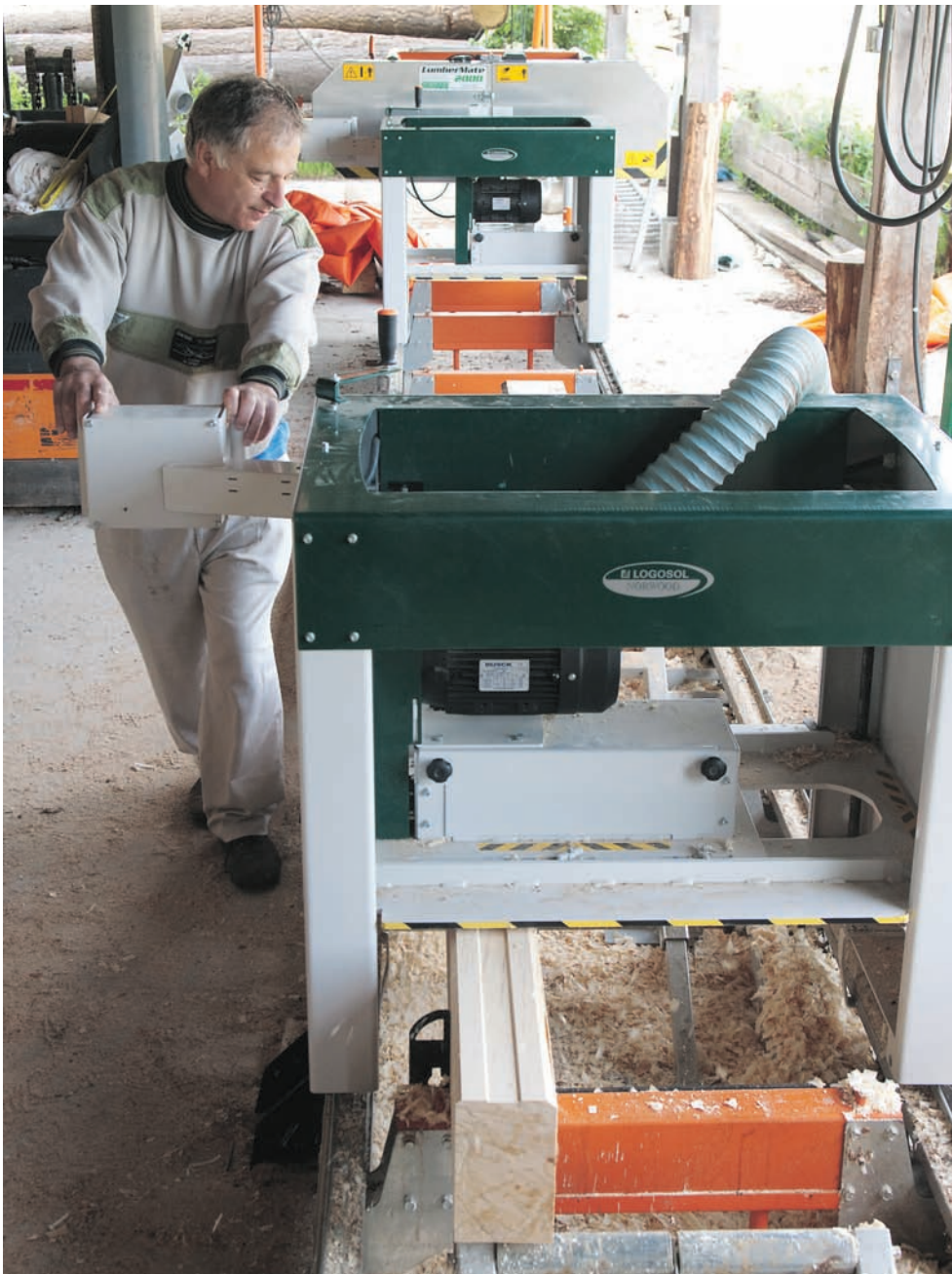
• Using two Log house Molders LM410, is a real time saver. One is for planing and the other one is for molding. "This saves much time", says Raymond.
