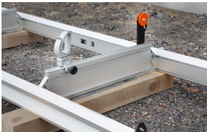
Sturdy log bed with a wide contact surface against the log.
